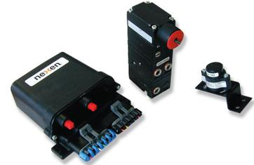
Nexen's innovative **dancer position control system** is ideal for out of round rolls, flying splice applications and multiple start/stop situations. The RSD100 Digital Dancer Controller maintains constant web tension with fast response to tension disturbances and features PC-based setup and calibration, eliminating potentiometer adjustments.
