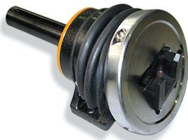
Nexen's line of rugged line of maintenance-free **safety chucks** provide roll shaft support and torque transmission at a low cost. Our product will safe-guard your equipment by securing the roll shaft in place during any wind or unwind operation. Nexen's safety chucks will only open with the socket in the upright position, and they are available in either foot or flange mounting.
