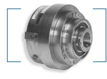
Nexen's 5HP-SE series: Spring-engaged tooth clutches provide the ultimate high torque holding in a small package when used as a brake. Mounting is simply a matter of fixing the pilot or drive flange to a stationary machine component. Spring-engaged tooth devices must be engaged at zero speed.
