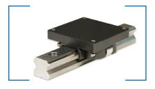
Nexen's RBR (rail brake roller) is a cost effective, light-weight solution for holding applications on guide rail systems. The unique design uses a horizontal air/spring chamber to apply force on the rail through a wedge and roller mechanism.
