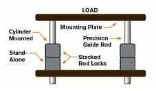
In vertical applications, multiple rod locks can be stacked to obtain a higher holding force.
