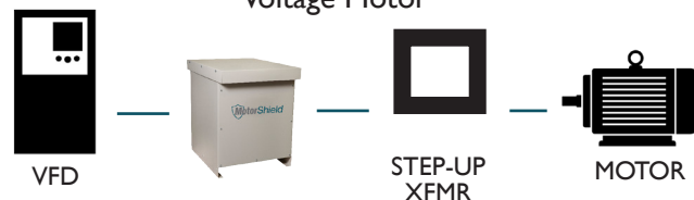
Low Voltage PWM Power Supply to Medium Voltage Motor
