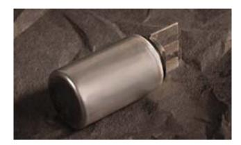
The Beta 1.5P building block is a Hall effect gear tooth sensor that accurately senses the movement of ferrous metal targets. It employs a specially designed Integrated Circuit, discrete components and a magnet that are enclosed in an environmentally sealed stainless steel can. This package has been carefully designed for cost-effective 2.0 level packaging.
