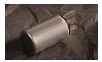
The 1.5P building block is a Hall effect gear tooth sensor that accurately senses the movement of ferrous metal targets. It employs a specially designed Integrated Circuit, discrete components and a magnet that are enclosed in an environmentally sealed stainless steel can. This package has been carefully designed for cost-effective final packaging.
