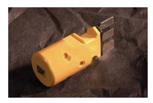
The 1.5M building block is a magnetoresistive gear tooth sensor that accurately senses movement of ferrous metal targets, both single or complementary. It employs a specially-designed integrated circuit and a magnet that are sealed into a probe-type package for physical protection and cost-effective installation into various applications.
