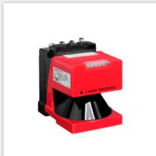
Contactless laser scanners for object detection and contour measurement. A laser measurement beam is deflected a rotating mirror and covers an area of 190° with a radius of up to 65 m. The measurement contour is output via Ethernet or a serial interface. In addition, there are models for object detection in up to four simultaneous detection fields.
