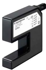
With mouth widths of 27 or 100 mm, this forked photoelectric sensor delivers accurate measurement results over a 25 mm long measurement range thanks to its CCD line. Depending on the configuration, it is possible to measure transparent edges, the diameters of wires, threads and much more.
