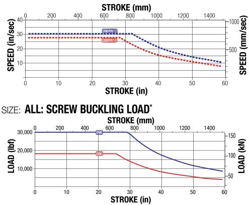
\*NOTE: When using Trunnion Mount, (TRR) consider the stroke to be longer when determining Critical Speed and Buckling Load:
