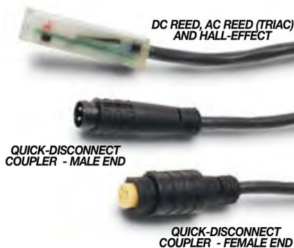
There are 10 sensing choices: DC reed, form A (open) or form C (open or closed); AC reed (Triac, open); Hall-effect, sourcing, PNP (open); Hall-effect, sinking, NPN (open); each with either flying leads or QD (quick disconnect). Commonly used to send analog signals to PLC (programmable logic controllers), TLL, CMOS circuit or other controller device. These switches are activated by the actuator's magnet.
