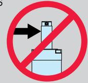
Measures are required, especially in "C" style designs, to limit side loading. For life optimization Tolomatic recommends side loads of less than 5% of axial load (thrust rod output force) for all roller screw configurations.
