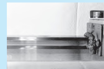
After the passage of ball slide (All contaminant particles are swept away)
