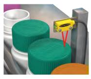
Bottle Cap Detection Using Fixed-Field Sensors
