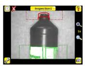
Multi-Point Inspection (Plus only) — Use seven to nine sensors in the same inspection
