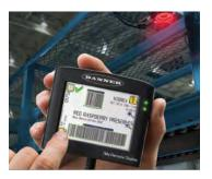
RD35 Handheld Remote Display Used for- programming
