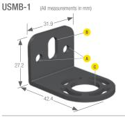
• Two-bracket replacement kit for brackets that come with emitter/receiver
