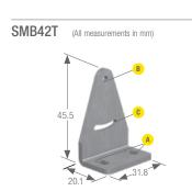
Hole center spacing: A = 20.3, B to C = 5.1Hole size:  $A = 4.3 \times 7.5$ ,  $B = \emptyset 3$ ,  $C = 3 \times 15.3$
