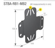
Hole center spacing: A = 20, B = 40, A = 20Hole size: (A), (B) = 27 x 7
