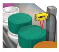
Bottle Cap Detection Using Fixed-Field Sensors
