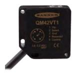
The QM42VT Vibration and Temperature Sensor makes it easy to monitor a machine's health. It measures RMS velocity (among other vibration characteristics) and temperature so that problems can be detected before they become too severe and cause additional damage or result in unplanned downtime. Paired with a Banner wireless Node, it can provide local indication, wirelessly send the signal to a central location, and send the vibration and temperature data to the Gateway for collection and trending.
