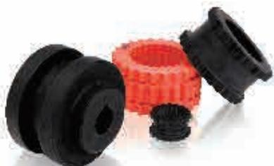
Three-way flexing action handles shock, vibration and misalignment. The ABB Dodge D-Flex™ coupling features moulded, non-lubricated, interchangeable elastomeric sleeves of EPDM, neoprene Hytrel. Its three-way flexing action accommodates torsional, angular and parallel misalignment, as well as axial end float.
