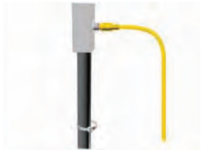
Moving Applications: Minimum bend radius 10x cable diameter
