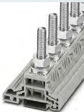
120 (120) mm², 269 A, M10 bolt terminal block
