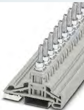
16 (16) mm², 76 A, M5 bolt terminal block
