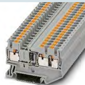
0.5 A, diode terminal block, 1N 4007 (1300 V/0.5 A), 3 connections
