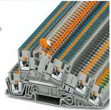
30 A, three-level terminal block, 1 x L outer conductor, 1 x N conductor can be disconnected, 1 x PE
