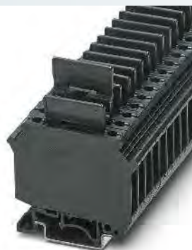
4 (4) mm², 6.3 A, fuse terminal block for 5 x 20 mm and 5 x 25 mm cartridge fuses
