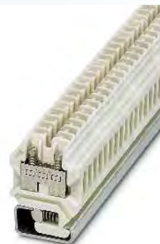
6 (10) mm 2 , 57 A, feed-through terminal block
