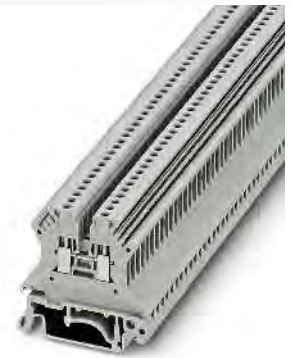
1.5 (1.5) mm², 17.5 A, feed-through terminal block
