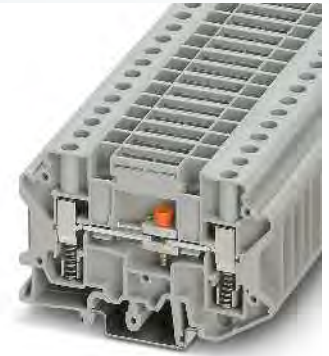
6 (10) mm², 57 A, test disconnect terminal block, for accommodating switching bridges, 2 connections
