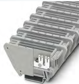
6 (6) mm 2 , 30 A, equipotential bond terminal block with spade connection
