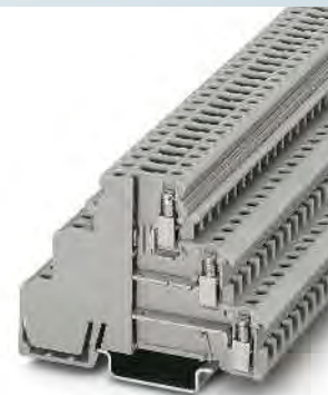
2.5 (4) mm 2 , 15 A, three-level terminal block with disconnect zone
