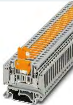
2.5 (4) mm², 16 A, knife disconnect terminal block with test socket screw
