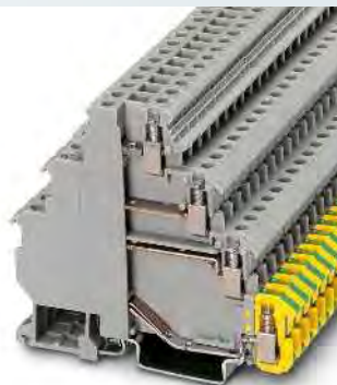
2.5 (4) mm², 26 A, four-level terminal block with PE foot
