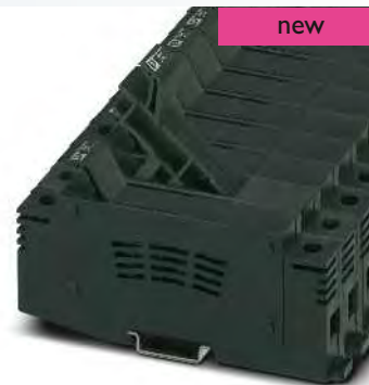
25 (25) mm 2 , 32 A, 1500 V, lever-type fuse terminal block for midjet fuses 10.3 x 85 mm
