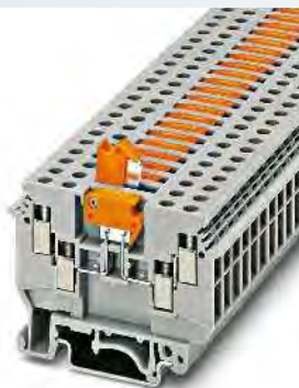
4 (6) mm², 16 A, knife disconnect terminal block, 4 connections, with test socket screw
