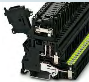
6.3 A, lever-type fuse terminal block for 5 x 20 mm cartridge fuses, with PE foot
