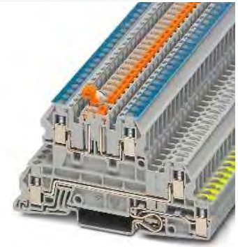
4 (4) mm², 24 A, three-level terminal block, 1 x L phase conductor, 1 x N conductor can be disconnected, 1 x PE
