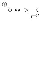
0.5 A, diode terminal block, 1N 4007 (1300 V/0.5 A), conducting direction: from left to right
