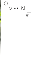
0.5 A, diode terminal block, 1N 4007 (1300 V/0.5 A), conducting direction: from right to left
