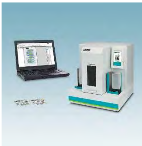
Direct laser marking
