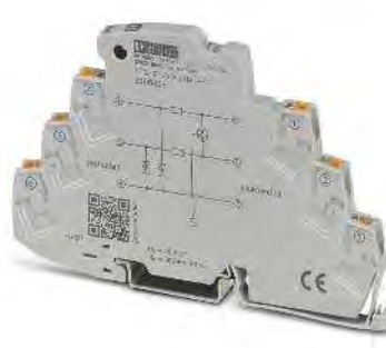
2-conductor with common reference potential, 3/6 connection grounded via gas-filled surge arrester, with or without status indicator and knife disconnection, e.g., for binary signals
