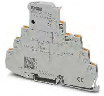
2-conductor with common reference potential, 3/6 connection grounded via gas-filled surge arrester, with knife disconnection, e.g., for binary signals
