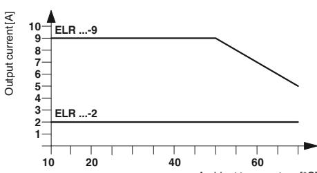
Load current as a function of the ambient temperature
