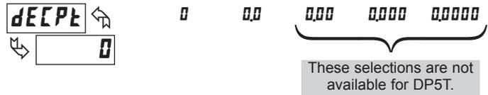
Select the decimal point location for the Input, MAX and MIN displays. (The TOT display decimal point is a separate parameter.) This selection also affects round, dSP 1 and dSP 2 parameters.
