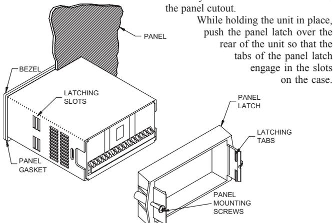
The panel latch should be engaged in the farthest forward slot possible. To achieve a proper seal, tighten the latch screws evenly until the unit is snug in the panel (Torque to approximately 7 in-lbs [79N-cm]). Do not over-tighten the screws.
