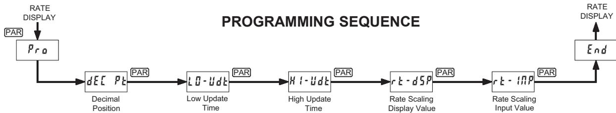
The Rate Indicator has five programmable parameters which are entered in the sequence shown above, using the front panel push buttons.
