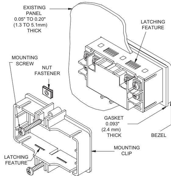
7. If the gasket is not adequately compressed and the mounting screws cannot be tightened any further, loosen mounting screws and insure that the clip is latched as close as possible to the panel.
