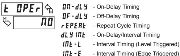
This parameter is used to select Predefined Operating Modes for the Timer. These modes cover a variety of timing applications frequently encountered in industrial control processes. When using a Predefined mode, the operator needs only to set the actual Setpoint On/Off or Time-out values for the particular application. However, each programming parameter will still be accessible, in order to make modifications to the predefined settings if desired.
