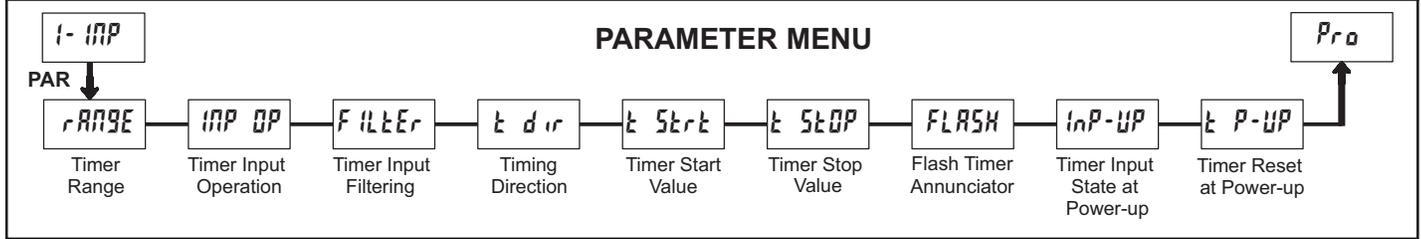
Module 1 is the programming module for the Timer Input Parameters. In the Display Mode, the TMR annunciator indicates the Timer display is currently being shown. An **EXCHANGE PARAMETER LISTS** feature, which includes the Timer Start and Timer Stop Values, is explained in Module 2.
