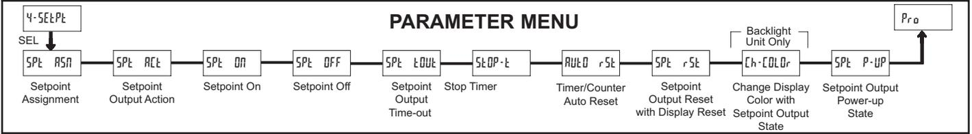
The Setpoint Output Parameters are only active when the optional relay module is installed in the meter. Some parameters will not appear depending on the Setpoint Assignment and Setpoint Output Action selected.
