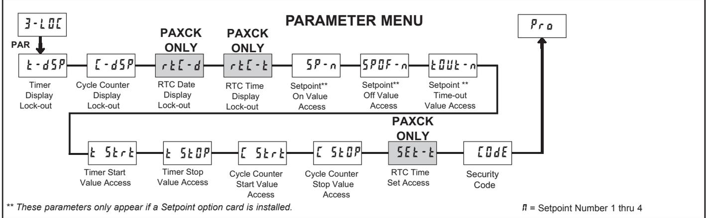
Module 3 is the programming module for setting the Display Lock-out Parameters and the “Quick Programming Mode” Value Access Parameters. In the Quick Programming mode, after the PROGRAM LOCKOUT PARAMETERS and before the Security Code (COdE), a Display Intensity Level (d-LEd) parameter is available when the security code is non-zero. It allows the display intensity to be set to 1 of 16 levels (0-15).
