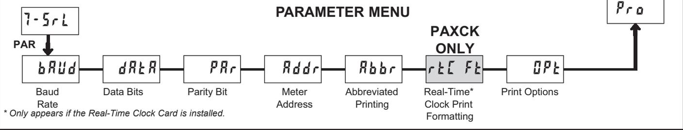
Module 7 is the programming module for the Serial Communications Parameters. These parameters are used to match the serial settings of the PAX with those of the host computer or other serial device, such as a terminal or printer. This programming module can only be accessed if an RS232 or RS485 Serial Communications card is installed.
