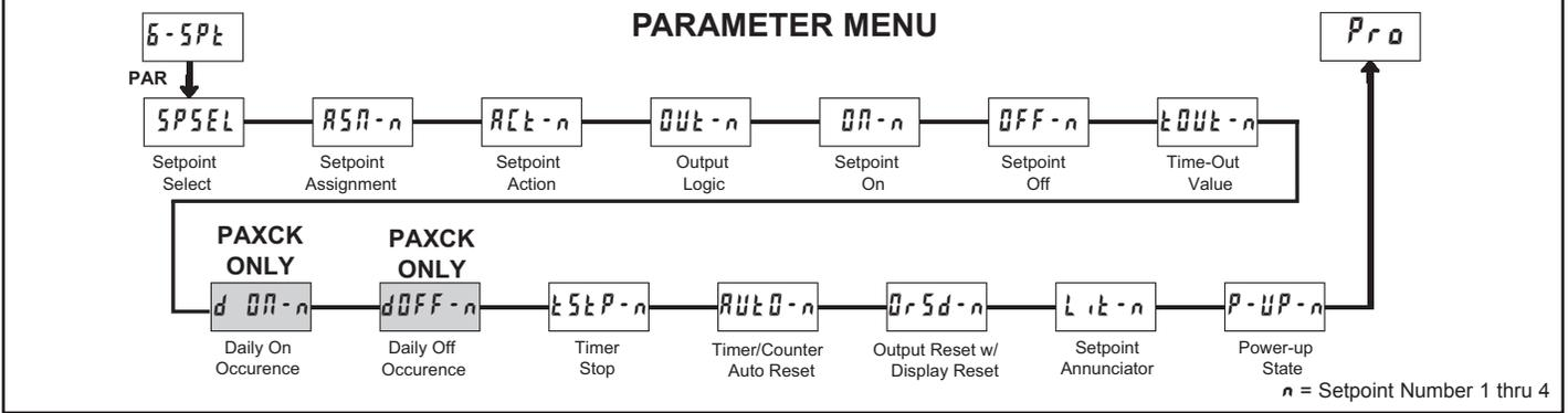
Module 6 is the programming module for the Setpoint (Alarm) Output Parameters. This programming module can only be accessed if a Setpoint card is installed. Depending on the card installed, there will be two or four Setpoint outputs available. The Setpoint Assignment and Setpoint Action parameters determine the applicable Setpoint features, and dictate which subsequent parameters will appear for the Setpoint being programmed.
