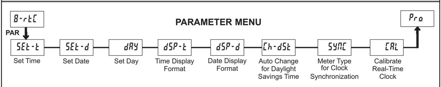
Module 8 is the programming module for the Real-Time Clock (RTC) Date and Time Parameters. In the Display Mode, the DAT annunciator indicates the RTC Date is currently being shown. The RTC Time display is shown with no annunciator. This programming module can only be accessed if a Real-Time Clock card is installed.
