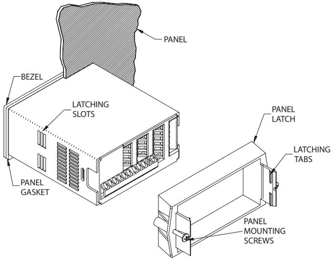
The meter should be installed fully assembled. Insert the meter into the panel cutout.
