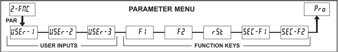
Module 2 is the programming module for the rear terminal User Inputs and front panel Function Keys.
