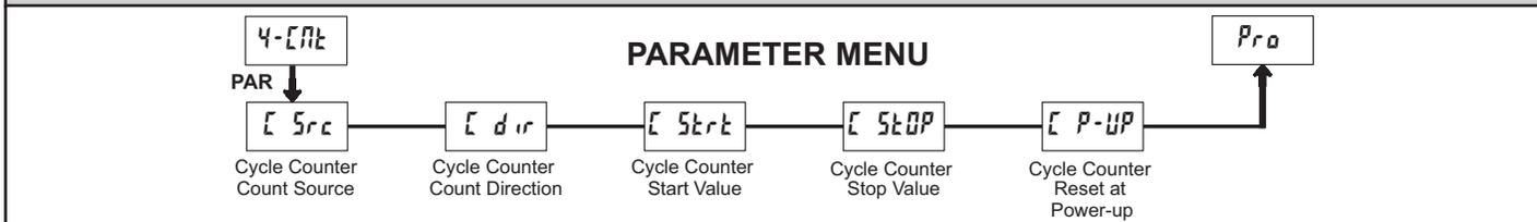
Module 4 is the programming module for the Cycle Counter Parameters. In the Display Mode, the CNT annunciator indicates the Cycle Counter display is currently being shown. An **EXCHANGE PARAMETER LISTS** feature, which includes the Cycle Counter Start and Stop Values, is explained in Module 2.
