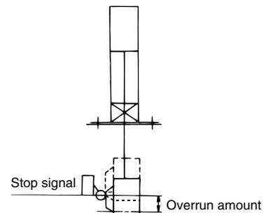
5. In order to further improve stopping accuracy, the time from the stop signal to the operation of the lock should be shortened as much as possible.
