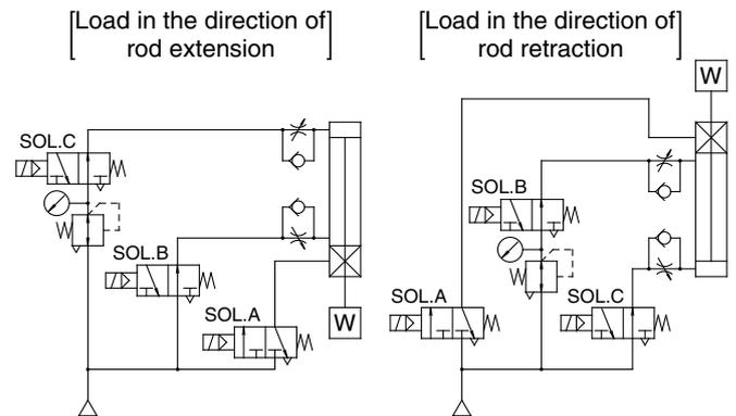
Note) The basic circuit examples are for spring locking (exhaust locking). For pneumatic locking (pressure locking) or spring and pneumatic locking, a 5 port solenoid valve should be installed in SOL.A.
