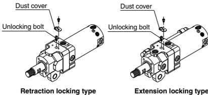
2. When the locking mechanism is to be used again, be sure to remove the unlocking bolt.
