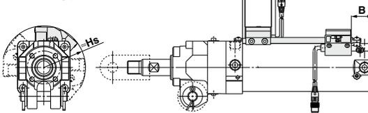
Note) The above drawing is the auto switch rod mounting example for the D-P49WSE type.
