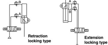
\* The symbol for the cylinder with lock in the pneumatic circuit uses SMC original symbol.
