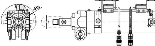
Note) The above drawing is the auto switch rod mounting example for the D-P4DWS□ type.
