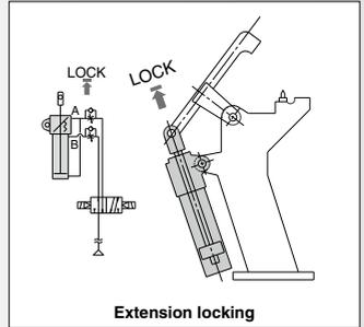
● Compact lock mechanism minimizes extension of length dimension.
