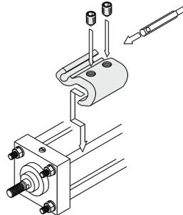
\* The above figure shows the mounting example of D-A9□(V)/M9□(V)/M9□W(V)/M9□A(V).
