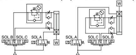
\* The symbol for the cylinder with lock in the basic circuit uses SMC original symbol.
