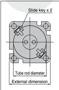
MGZ series employs a slide bearing and a large bore tube rod that accounts for approximately 80% of the cylinder's external diameter. In addition, a built-in non-rotating mechanism using slide keys allows loads to be mounted directly.
