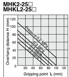
(Note) Distance to the gripping point L of single acting type is shortened by spring return.
