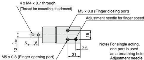
Note) For single acting, one port is used as a breathing hole. Adjustment needle for finger speed is used as a plug.
