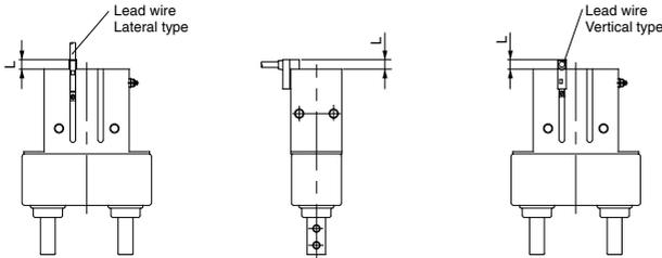
Note) When auto switch for MHK2, MHKL2 is set on mounting side as figure below, allow for at least 1 mm on mounting plate since the auto switch is protruded from edge of gripper.
