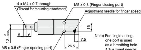
Note) For single acting, one port is used as a breathing hole. Adjustment needle for finger speed is used as a plug.
