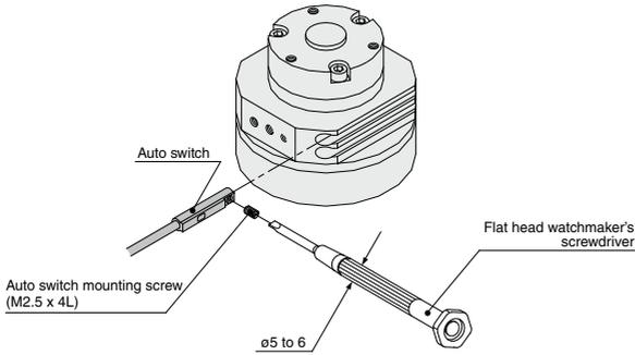
Note) Use a watchmaker's screwdriver with a grip diameter of 5 to 6 mm to tighten the auto switch mounting screw. The tightening torque should be about 0.05 to 0.15 N·m.
