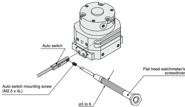
Note) Use a watchmaker's screwdriver with a grip diameter of 5 to 6 mm to tighten the auto switch mounting screw. The tightening torque should be about 0.05 to 0.15 N·m.
