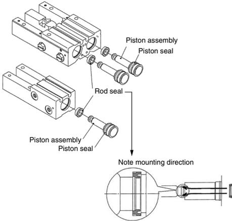
5. Apply the specified grease lightly to the sliding interface between the outer periphery and the body of the piston, and assemble them in the reversed order.
