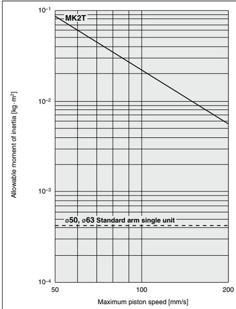
Note) Maximum piston speed is equivalent to approximately 1.6x the average piston speed. (Rough indication)
