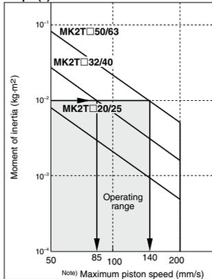
When arm's moment of inertia is  $1 \times 10^{-2}$  kg-m<sup>2</sup>, cylinder speed should be less than
