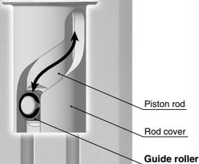
Non-rotating accuracy:  $\pm 0.9^\circ \Rightarrow \pm 0.5^\circ$
