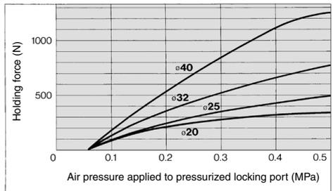
1. The holding force is the lock's ability to hold a static load that does not involve vibrations or shocks, after it is locked without a load. Therefore, to use the cylinder near the upper limit of the constant holding force, be aware of the following:
