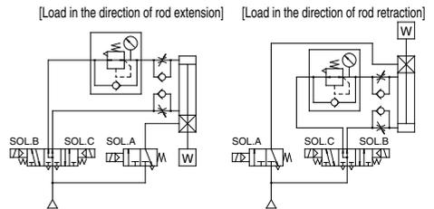
\* The symbol for the cylinder with lock in the basic circuit uses SMC original symbol.
