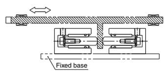
Using two MQP cylinders can improve the thrusting accuracy of an MQQ and/or MQM double acting metal cylinder. Additionally, equal strength of both extension and retracting thrust can be obtained.
