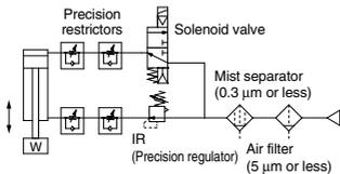
\* When using a solenoid valve, use a metal seal type (VQ, VQZ, SQ series, etc.).
