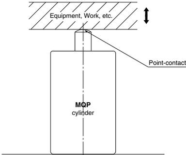
The material of the cylinder rod is heat-treated stainless steel (HRC60). The roughness of the spherical contact of the attaching part (Equipment, Work, etc) should be Rz6.3 and the material should be HB100 or greater (Aluminum material: 2000 line or 7000 line or equivalent) When higher precision or longer service life is required, we recommend using a heat-treated material + flat polished machined material (Rz0.8)
