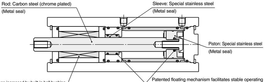
Lateral load resistance increased by built-in ball bushing
