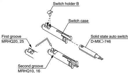
3. Install the auto switch case, with a switch attached securely in the hole, in the direction indicated in Figure (1).
