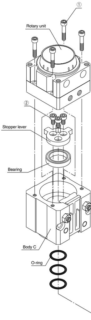
1. Loosen the four bolts ① and remove the rotary unit.
