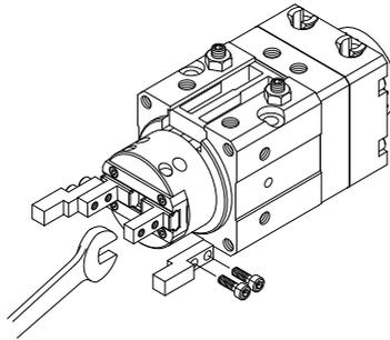
When mounting attachments on fingers, support the fingers with a tool such as a spanner to prevent them from twisting. Refer to the table on the right for the tightening torques of finger mounting bolts.
