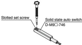
2. Insert the auto switch into the switch case, and install switch holder B into the first groove (MRHQ20/25) or the second groove (MRHQ10/16) and secure the auto switch.
