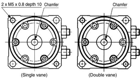
The outside drawings show the single vane type, but only the position of the chamfered sections shown in the above drawings differs from single and double vane.
