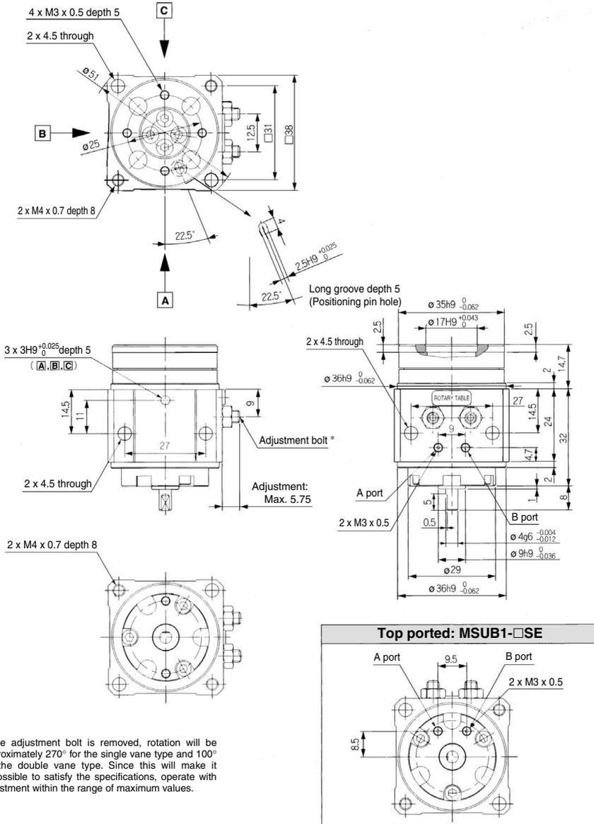
\* If the adjustment bolt is removed, rotation will be approximately 270° for the single vane type and 100° for the double vane type. Since this will make it impossible to satisfy the specifications, operate with adjustment within the range of maximum values.
