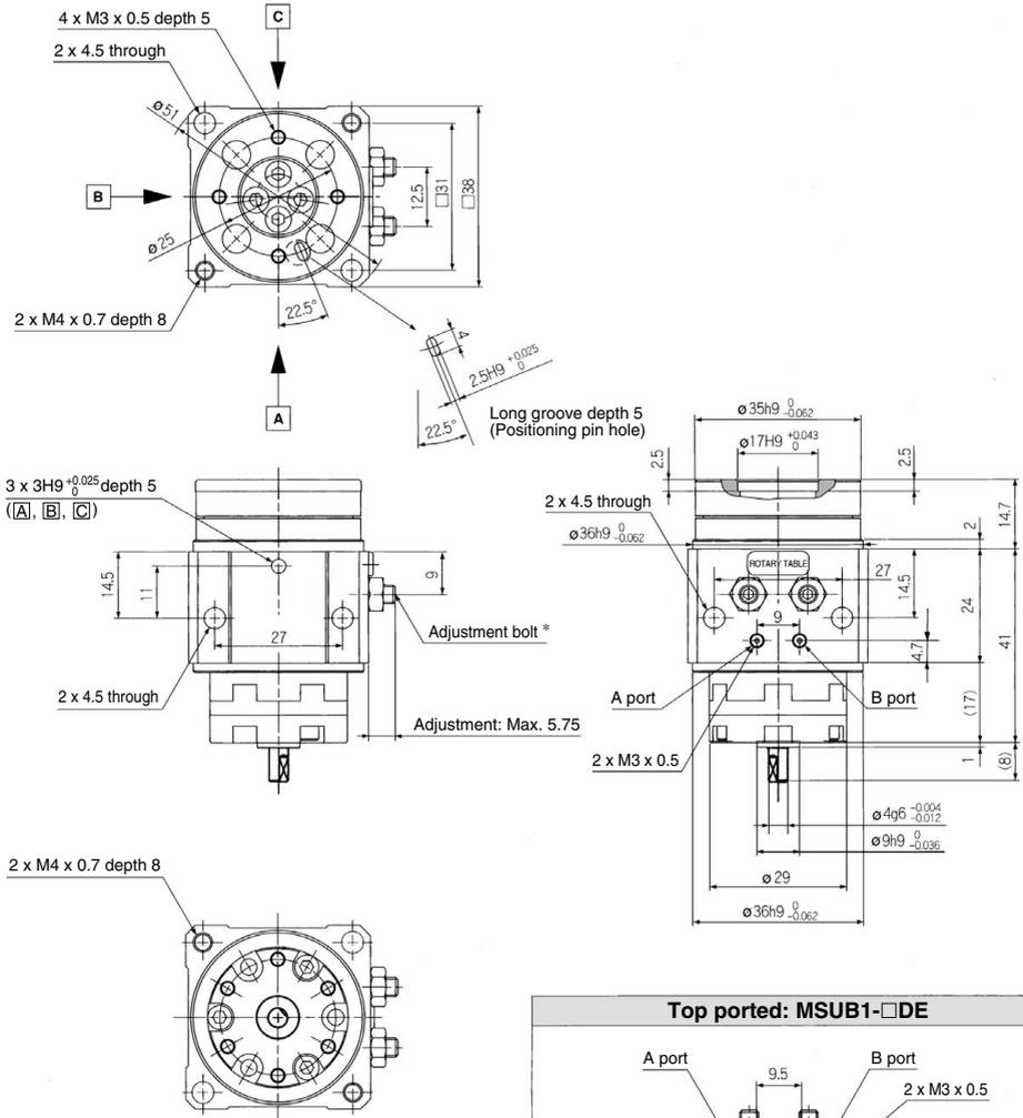
\* If the adjustment bolt is removed, rotation will be approximately 270° for the single vane type and 100° for the double vane type. Since this will make it impossible to satisfy the specifications, operate with adjustment within the range of maximum values.
