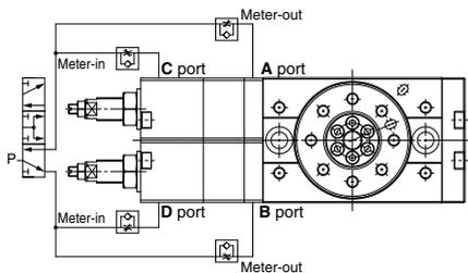
**Figure 2** 3-position solenoid valve: 2 pcs.
