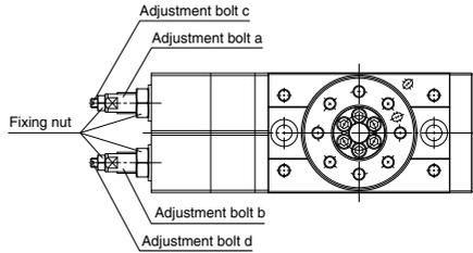
**Figure 5** Angle adjustment Range
