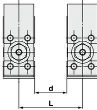
Dimensions of a shielding plate (MU-S025) that is sold separately are indicated as reference.
