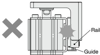
3. Do not apply strong impact or an excessive moment while mounting a workpiece.
