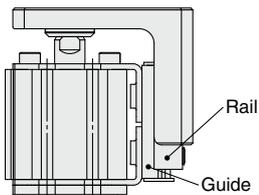
6. Do not remove the bolts holding the linear guide when removing the product. Incorrect handling of the product may cause mounting accuracy failure.
