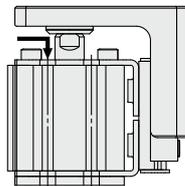
(2) When mounting an auto switch into the groove from the top
