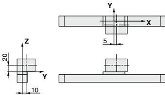
**Workpiece Mass and Center of Gravity**
