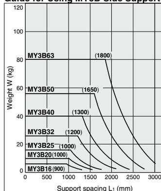
Note) A side support must be used to keep the spacing from exceeding the value inside the parentheses.
