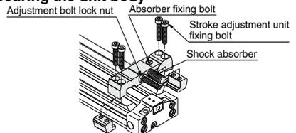
Tighten the four unit fixing bolts equally to secure the unit body.
