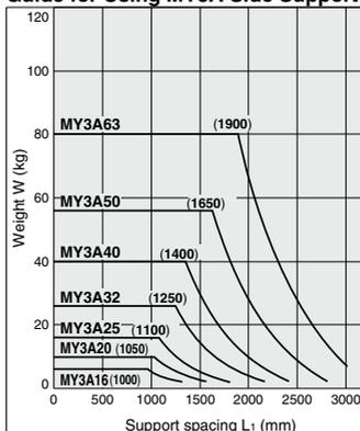
Note) A side support must be used to keep the spacing from exceeding the value inside the parentheses.
