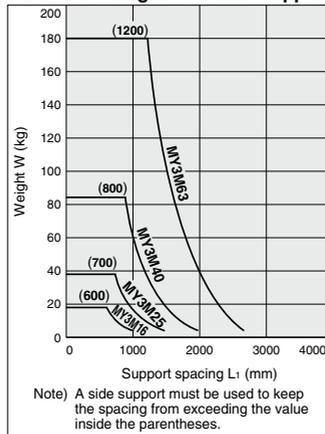
Note) A side support must be used to keep the spacing from exceeding the value inside the parentheses.
