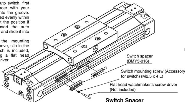
Note) Use a watchmaker's screw driver with a handle diameter of 5 to 6 mm to fasten the auto switch mounting screws. The tightening torque should be approximately 0.1 to 0.15 N·m. The guideline is a 90° rotation after the fastening is felt.
