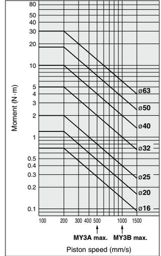
Select the moment from within the range of operating limits shown in the graphs. Note that the maximum allowable load value may sometimes be exceeded even within the operating limits shown in the graphs. Therefore, also check the allowable load for the selected conditions.
