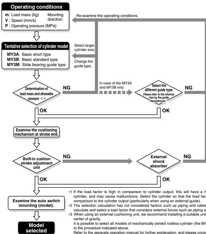
\*1 If the load factor is high in comparison to cylinder output, this will have a negative affect on the cylinder, and may cause malfunctions. Select the cylinder so that the load factor is less than 0.5 in comparison to the cylinder output (particularly when using an external guide).
