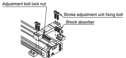
Tighten the four unit fixing bolts equally to secure the unit body.
