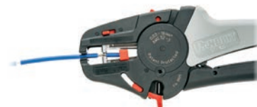
Step C Complete Stripped wire
