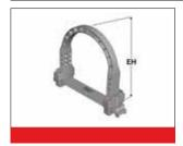
Large-diameter conduits are routed securely by using bracket bars (BS). This bar is installed on the crossbars or the covers of the cable drag chain. The bracket bar can be installed on both the inside and outside bend.
