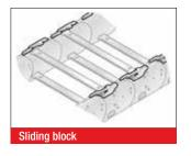
In the case of cable drag chains, sliding blocks are used in a horizontally sliding installation mode (the tight side of the chain slides on the slack side). The sliding blocks are set onto the side links on the interior bend instead of the usual crossbar interlocks; (no tools needed). This forces the chain to slide on the sliding blocks instead on the side links of the chain. Depending on the application, the service life of the cable drag chain may be extended five-
