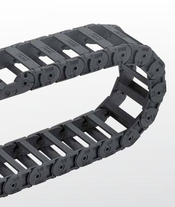
ORDERING EXAMPLE: 0140 01 020 048 0 0 988 Crossbar in inside and outside bend; can be opened in outside bend Inside width 0.79 in. (20.00 mm); 1.89 in. (48.00 mm) Full-ridged with bias, material black-colored polyamide Chain length 38.9 in. (988.00 mm) (38 links)
