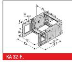
This chain bracket offers universal connection options (top, bottom and front) and is attached to the ends of the chain like a side link. This allows the chain to move right up to the bracket. Each chain requires one male and one female bracket. M5 screws are used to secure the brackets in place. Extrusion-coated metal bushes with either a through-hole (-FB) or a threaded hole (-FG) ensure the permanent, high-strength transmission of even extreme forces onto the cable drag chain.
