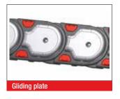
The gliding plates are mounted in a horizontal position, with the chain laying on its side, to minimize friction wear to the sides. They are mounted to the side links using a special screw. v We recommend replacing the cable drag chain when this limit has been reached. Depending on the application, the service life of the cable drag chain may be extended two-fold, by using gliding plates. The cable drag chain must be placed on its side before opening.
