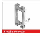
For crossbars wider than 9.69 inch (246 mm), we recommend the use of crossbar connectors. These prevent deformation to the crossbar under large amounts of additional weight of the chain assembly.
