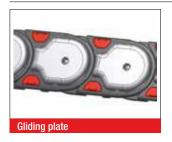
The gliding plates are mounted in a horizontal position, with the chain laying on its side, to minimize friction wear to the sides. They are mounted to the side links using a special screw. The wear limit is 0.1 in (2.5 mm). We recommend replacing the cable drag chain when this limit has been reached. Depending on the application, the service life of the cable drag chain may be extended two-fold, by using gliding plates. The cable drag chain must be placed on its side before opening.
