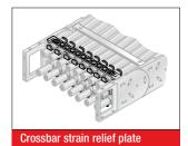
Fixed integrated crossbar strain relief plates in the chain brackets. Tailored to all crossbar widths up to 9.69 inch (246 mm). May be assembled on the inside and outside bends at both chain endings.
