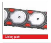
The gliding plates are mounted in a horizontal position, with the chain laying on its side, to minimize friction wear to the sides. They are mounted to the side links using a special screw. The wear limit is 0.1 in (2.5 mm). We recommend replacing the cable drag chain when this limit has been reached. Depending on the application, the service life of the cable drag chain may be extended two-fold, by using gliding plates. The cable drag chain must be placed on its side before opening.
