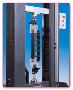
Murrplastik cable drag chains have been developed for use in extreme conditions. The standard material is glass fibre reinforced plastic in standard black.
