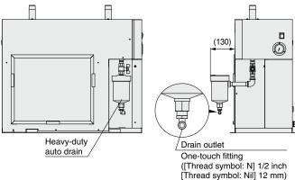
\* The heavy-duty auto drain and piping materials (nipple, elbow) are shipped together with the main body of the air dryer. Customers are required to mount the parts to the air dryer.
