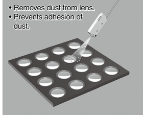
Neutralizing static electricity from lens
