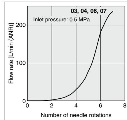
\* The numbers above the flow rate characteristic curves in the charts show the applicable tubing outside diameter as defined by the product number.
