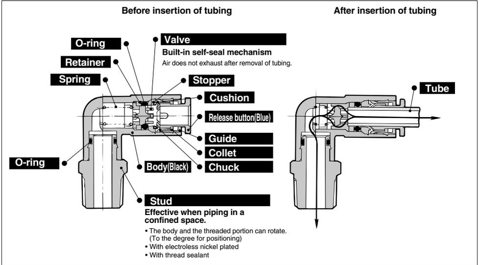
**One-touch fitting (built-in self-seal mechanism) to prevent air exhaust when removing tube.**
