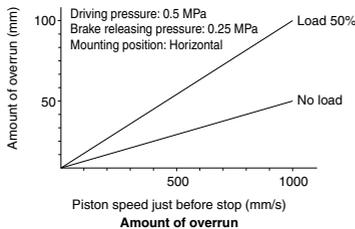
The graph above shows the relation between piston speed and overrun. (The length of overrun is changed, dependent on piston speed, load, piping conditions and control method. Be sure to adjust the stop signal position, etc. by trial operation with the actual machine.)
