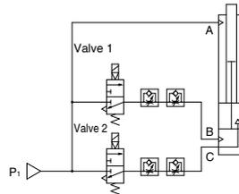
Return to the retraction end when power supply is stopped
